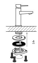
4. PLACE NEW FAUCET IN THE POSITION ON THE SINK. FROM UNDER THE SINK, PUT GASKET AND METAL PLATE AND THREAD NUT ONTO THE PIN. TIGHTEN THE NUT. PLACE SET SCREWS IN TO THE NUT AND TIGHTEN THEM.
