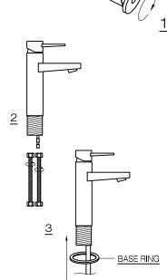
2. CONNECT FLEXIBLE HOSES TO THE BRASS PIPES.
